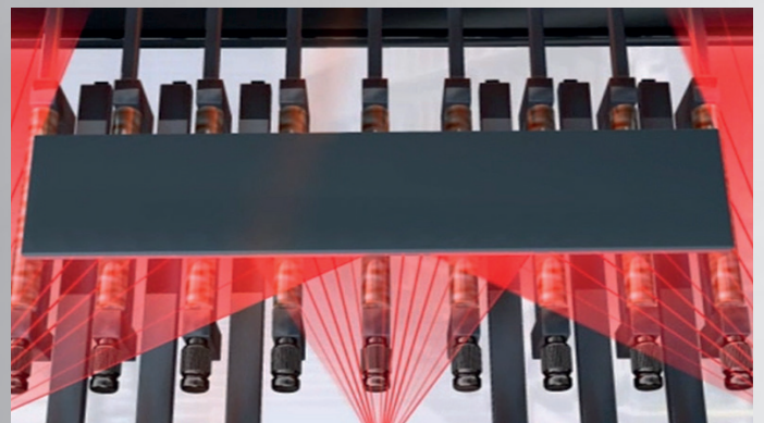
Function principle of the slab positioning at the roller table
