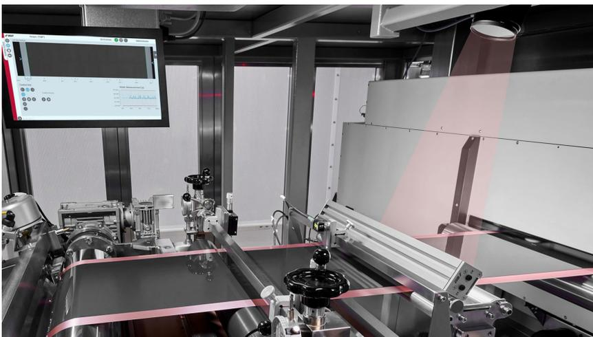
Even small imperfections in battery manufacturing result in rejects. BST COATINGControl® provides a decisive competitive advantage by enhancing plant efficiency: To achieve flawless coating geometry on front and back, the system employs high-precision measurement and control technology.
