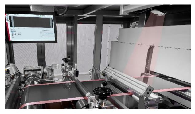
((BST COATINGControl.jpg)) BST COATINGControl combines intelligent control technology and precise measuring instruments to automatically optimize web running processes.
