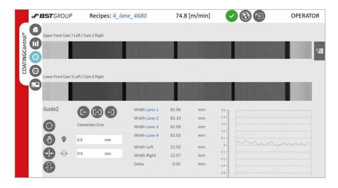
((BST\_COATINGControl\_Bedienoberfläche.jpg)) BST COATINGControl provides comprehensive, intuitive, mobile and precise information on all relevant parameters: a live image of both coating sides. Optionally, the user interface can be accessed on mobile devices.
